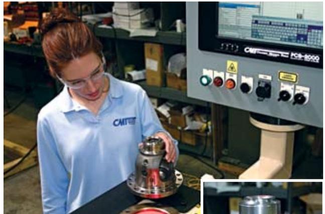
In the application shown, the UID/2D pulsed-laser marking machine uses a new 20w Sun Matrix high-speed fiber laser marking head to permanently mark 2-D matrix codes and part numbers on rough machined surfaces of cast iron automotive differential cases.
