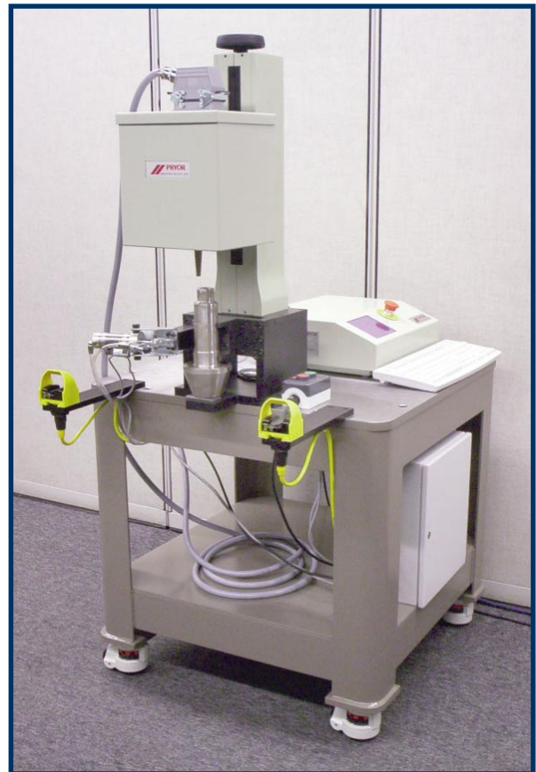
Marking pinion shaft (overall system)
